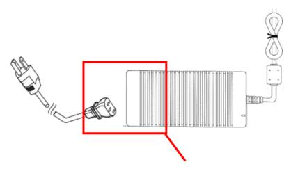
Unplug the power cord from the power adapter jack to disconnect the device.
